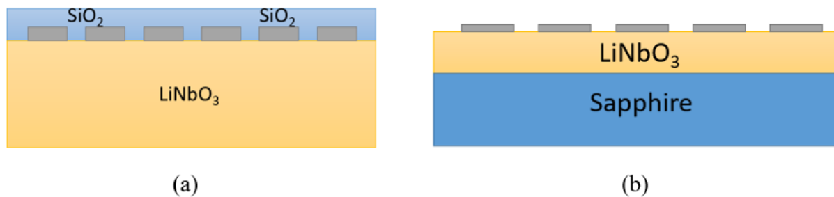
Figure 5.18 Temperature compensation techniques used in piezoelectric acoustic resonators: (a) thin film overlay; (b) thermal expansion constraint.
